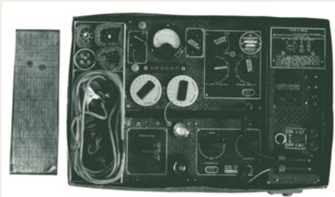
The Type 3 Mk II (R2) radio set (Type 3) The most widely used set from 1942/3 through to 1945. A very good set, able to operate with a power supply of 20 watts, capable of being used from AC/DC mains or batteries - it could be swapped over from mains to batteries simply by reversing a plug on the power unit which would operate from 27-220 volts AC. The main set above is shown in a suitcase. Below illustrates the set in their portable container as they would have been if dropped to the Resistance.
